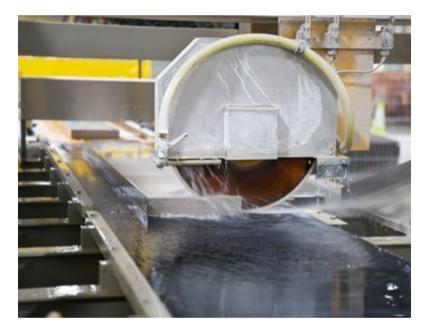
Recycling water is reused several times into the manufacturing process and is compulsory to achieve ANSI 373 Standard.
