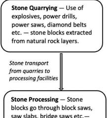
saw slabs, bridge saws etc. stone blocks processed to stone flooring and paving products.
