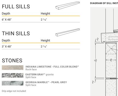
DIAGRAM OF SILL INSTALLATION
