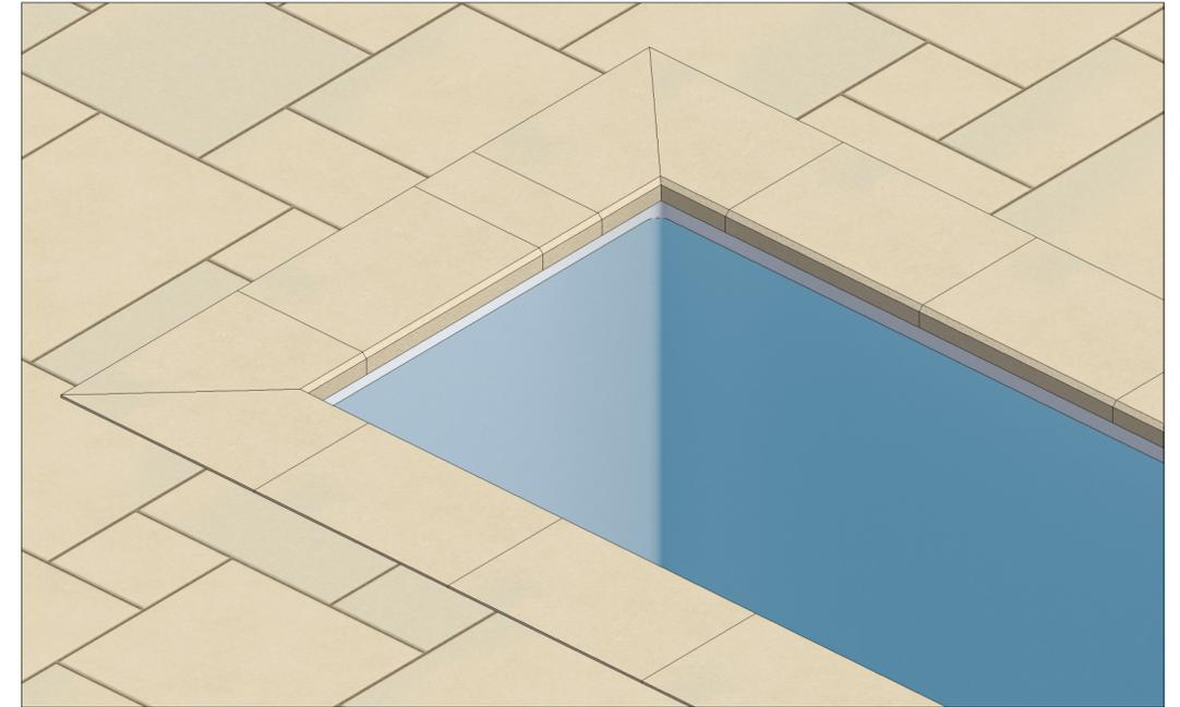
**POOL COPING - CHAMFERED EDGE - 12" x 24" x 2"**
